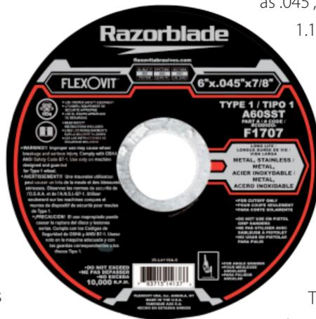
The third and final number in the example [7/8"] represents the arbor size. This is the only measurement that is a true representation of the actual size as measured as it is dictated by ANSI B 7.1-2000 "Safety Requirements for the Use, Care, and Protection of Abrasive Wheels". ✦
